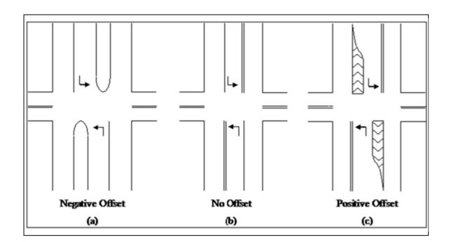
A *negative offset* places the left turning vehicles in direct eyesight of each other resulting in an obstruction of the sight triangle. The left turning vehicles are unable to see oncoming through traffic.
